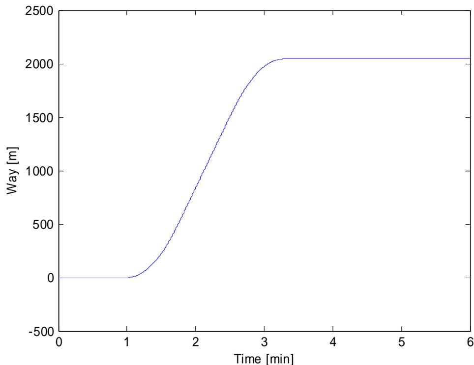
After one minute stop-time at Ringlikon, the end-station Uetliberg is reached after 3,5 minutes. On the time schedule, 6 minutes between stop in Ringlikon and Uetliberg are reserved: two minutes reserve remains.
