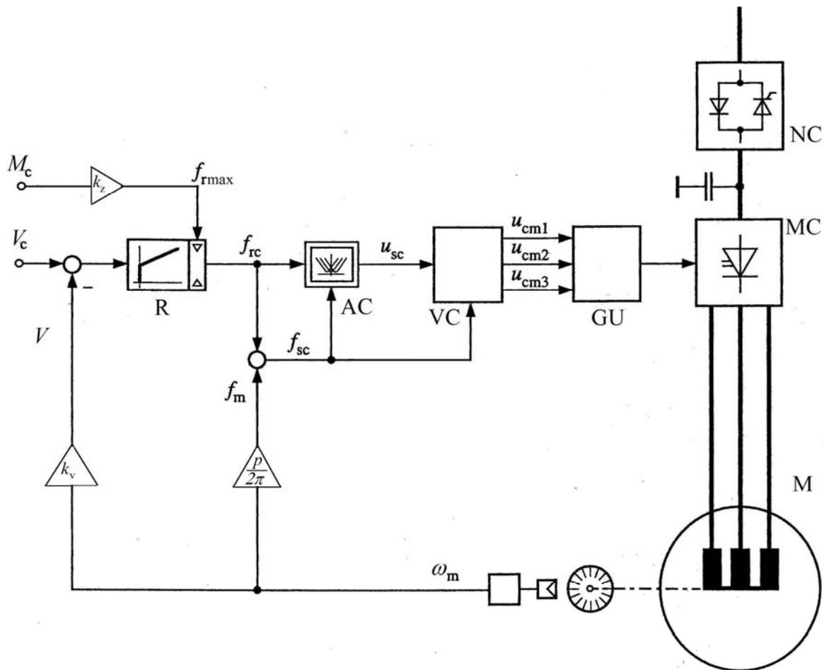
The network converter NC is controlled by a controller – not represented on the figure – which holds a quite constant value at the voltage intermediate circuit.
