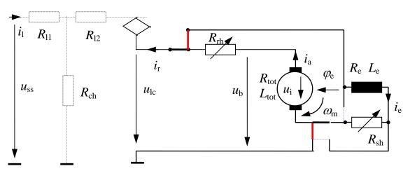
Fig. 4.17 DC-motor with separate excitation: principle of regenerative braking.
