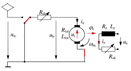
Fig. 4.13 DC-motor: rheostatic braking with separate excitation.
