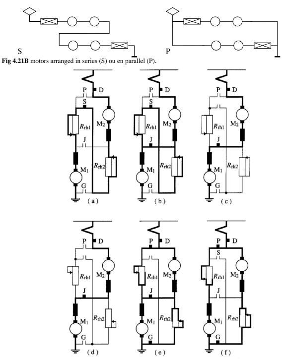
Fig. 4.22 Sequence from steps in a series-parallel transition with bridge-method (BOB : ABeh 4/4 II).
