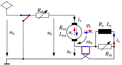
Fig. 4.4 Motor series in traction.
