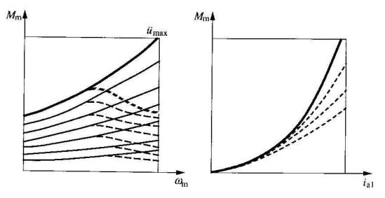
Fig. 4.61 Regenerative braking with separate excitation: characteristics.
