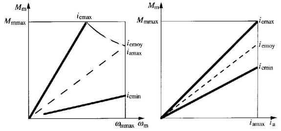
Fig. 4.50 Rheostatic braking at DC-excitation: characteristics.
