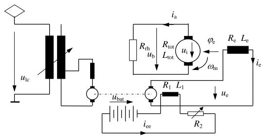
Fig. 4.46 & 4.48 Rheostatic braking at DC-excitation: diagram with generator group.
