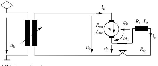
Fig. 4.42 Series motor in traction.
