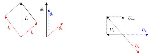
Fig. 4.38 & 4.39 Commutation in single-phase motor without and with ohmic shunt.
