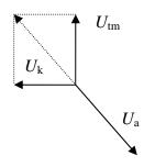
Fig. 4.40 Commutation in single-phase motor at low or nominal speed.
