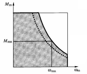
Fig. 4.164B Induction motor and three-phase converter: characteristics versus speed.
