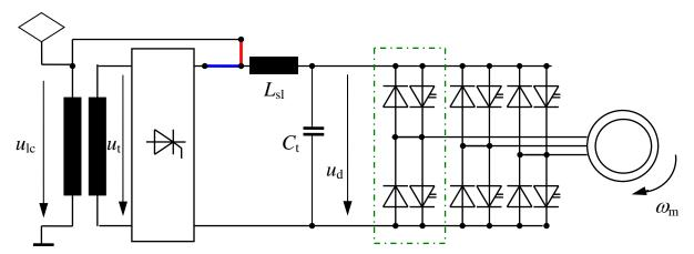
Fig. 4.164A Induction motor and three-phase converter for DC- or AC-contact line. Principle drawing.
