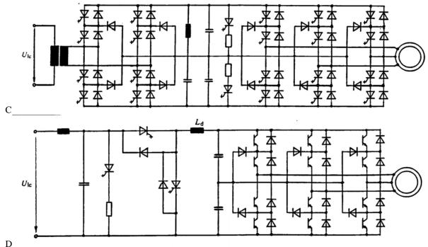
Fig. 4.166 C Bidirectionnal U-converter with GTO for AC contact line GTO (CFF : Re 460).D Bidirectionnal U-converter with IGBT for DC contact line (JNR : 207).
