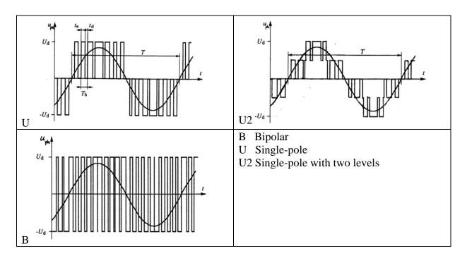
Fig. 4.168 Inverter arm-control.
